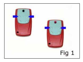
3) Place the remote to clone from, (in this case the blue remote) head to head as shown in and press the button you want to copy. The LED on the copying remote (red) goes out, indicating it has copied from the blue remote successfully. (You only have 15 seconds to do this step)
