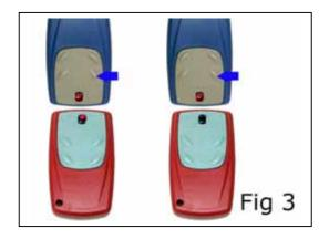
2) Press once the spare button that you want to programme, the LED stops flashing and stays on indicating it is ready to accept a code.
