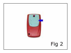
3) If the LED on the cloning remote fails to go out straight away, try passing the transmitting remote underneath the remote to be cloned as shown. The LED only stays on solid for 15 seconds to accept a code after which it times out.
